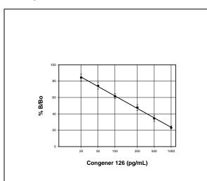
**Coplanar PCB Standard Curve**
