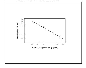
Water samples containing PBDEs within the dynamic range (25-1,000 ppt) can be directly tested in the assay after filtration.
