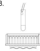
Add 1 mL of Washing Solution down the inside wall of each tube by using the technique described in Box 2. Wait 2 minutes. Using a smooth motion, invert the combined rack assembly over a sink and pour out the tube contents: keep inverted and gently blot the test tube rims on several layers of paper toweling. Repeat this step.
