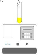
Add 500  $\mu L$  of Stopping Solution down the inside wall of each tube by using the technique previously described. Read results at 450 nm within 15 minutes after adding the Stopping Solution. Multiply results of samples by the appropriate dilution factor (if any).
