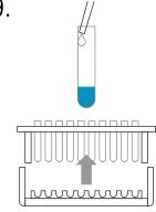
Lift the upper rack (with its tubes) off the magnetic base; add 500 µL of Color Reagent down the inside wall of each tube by using the technique described in Box 2. Vortex for 1 to 2 seconds (at low speed to minimize foaming).
