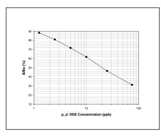
Samples containing DDDE within the dynamic range (1.25-75.0 ppb) can be directly tested in the assay after filtration (if necessary).
