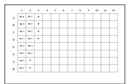
Add 25 μL of the appropriate standard or sample to the wells of the test strips according to the working scheme shown above. Analysis in duplicates or triplicates is recommended.
