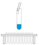
Add 500 µL of Color Reagent down the inside wall of each tube by using the technique described in Box 2.
